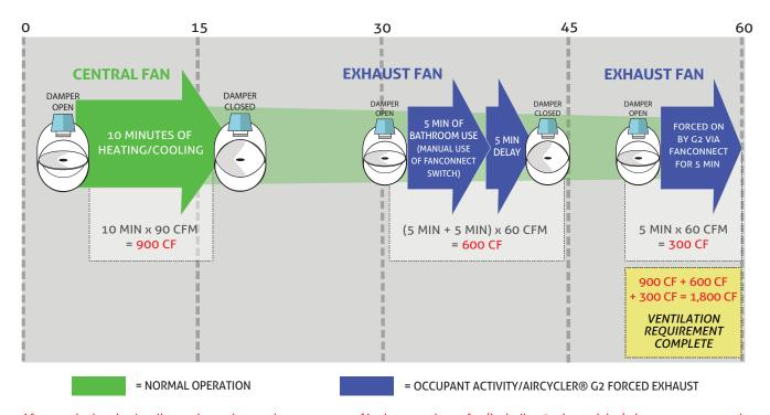
After regular heating/cooling cycles and manual occupant use of bathroom exhaust fan (including 5 minute delay), there was not enough ventilation to meet requirements for the hour. At the end of the hour the AirCycler® g2 forced on the bathroom exhaust fan, via the FanConnect™ switch, to reach required ventilation.
