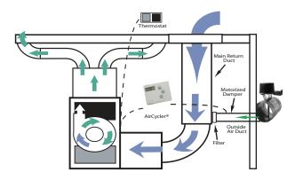
\* Upon system startup be sure to set damper power switch to UP or AUTOMATIC position
